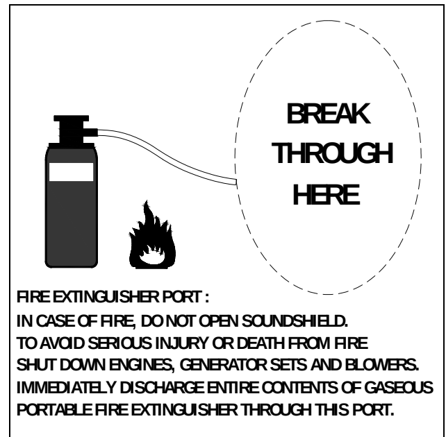
Fig. 2: Fire extinguisher port.
